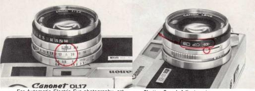
For Automatic Electric Eye photography, set the aperture ring at "A" position.
